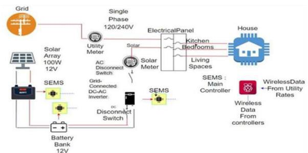
Figure-1: Block Diagram of General SHEMS Architecture (Courtesy: Internet)
