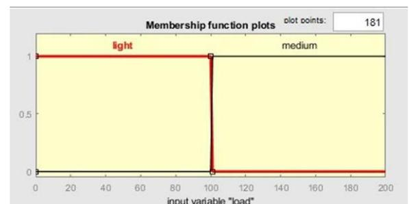
Figure-4: Membership function for input variable Load
