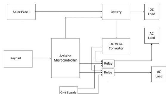
Figure-2: Block Diagram of Proposed SHEMS Framework
