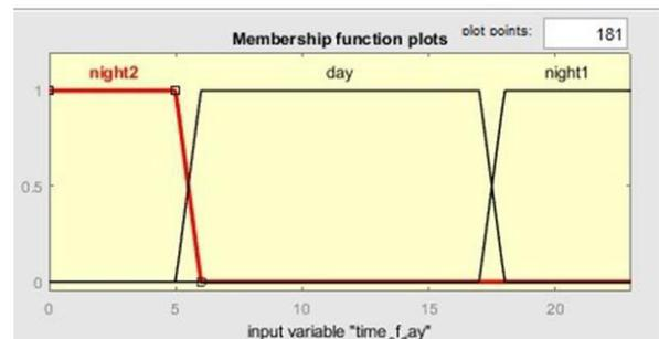
Figure-3: Membership function for the input variable Time
